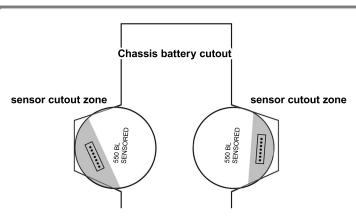
• Position 550 sensored motors with the sensor plug on the outside of the battery in the sensor cutout zones. Shorter motors generally do not have mounting requirments and can be rotated in any position as long as they clear your battery. • The battery can be moved out by changing spacer lengths or locations of the retaining system.
