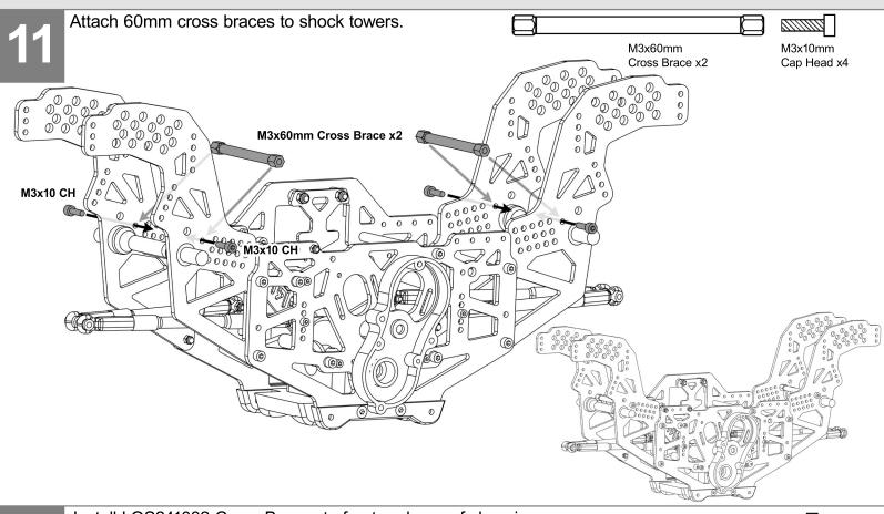
Install LOS241032 Cross Braces to front and rear of chassis. If using Team PRP Duo towers you can attach Losi LMT body posts in either location shown using the body post hardware from your LMT kit.
