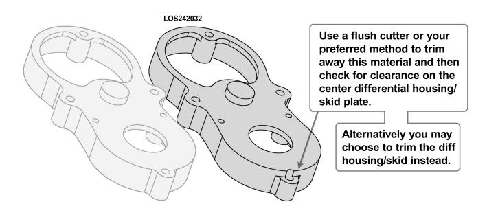
Install Gearbox Housing to right side chassis plate. Choose fore or aft motor weight bias position.
