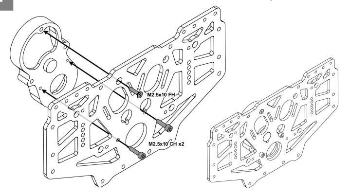
Assemble battery retaining system.
