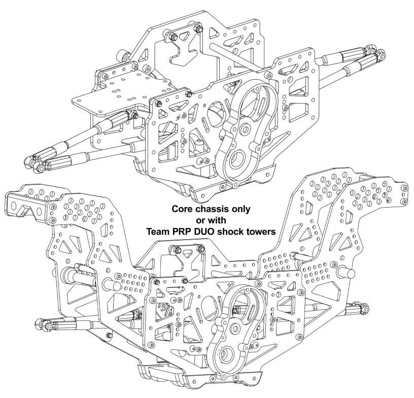
Chassis conversion for the Team Losi LMT RTR, Roller, or TLR Tuned trucks. Single motor, lower center of gravity 2S shorty side mounted battery and fore or aft weight bias tuning with motor and electronics position options.
