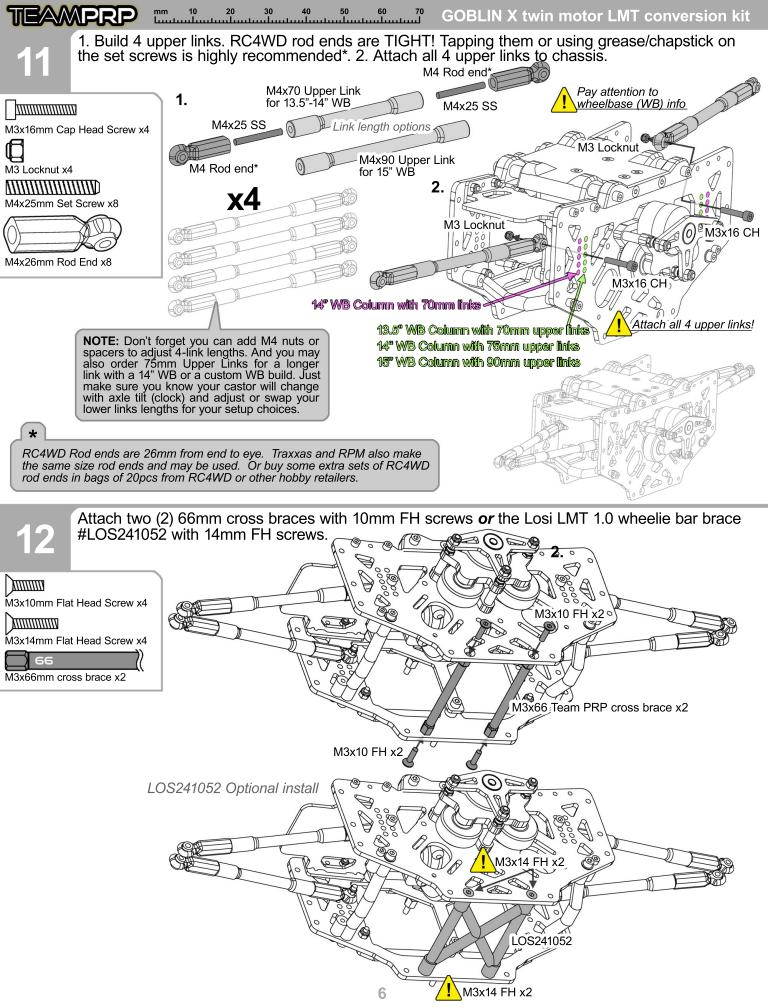
Attach the lower links from your Losi LMT donor kit or custom setup. Lower links are not included with the Goblin X kit as you generally use the links from the donor kit you are converting from. See link notes below.
